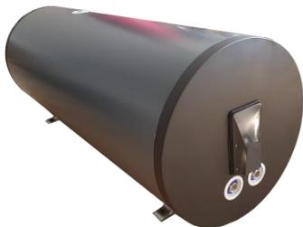
The storage tank consists of an outer chromadek wrap with two powder coated end caps. Within this wrap is an inner steel tank which is insulated from the outer wrap by polyurethane foam. The inner tank is made from 316 stainless steel. There are 5 x 20mm female ports for plumbing connections.
