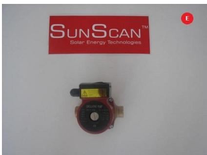
The GPD20-6SB 220v single phase brass bodied circulation pump is 3 speeds adjustable and capable of circulating 18lpm-50lpm (3000lph on max setting).
