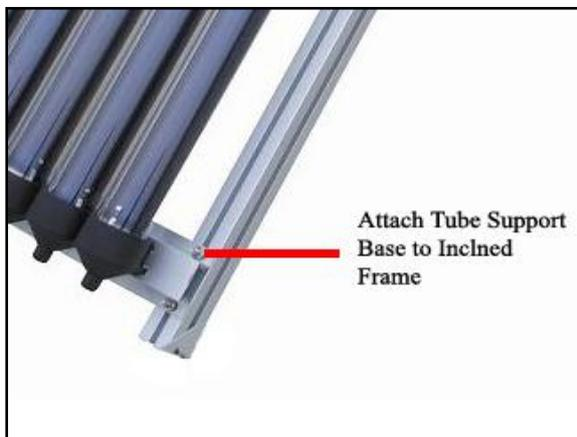
Place the tube support base on the bottom of the inclined tracks. Lightly bolt it to the front tracks using the brackets and bolts provided. Adjust the distance between the manifold and the tube support base by inserting a tube in the manifold and securing it in the tube support base. Refer to section below for the procedure. Tighten the bolts to secure the tube support base.
